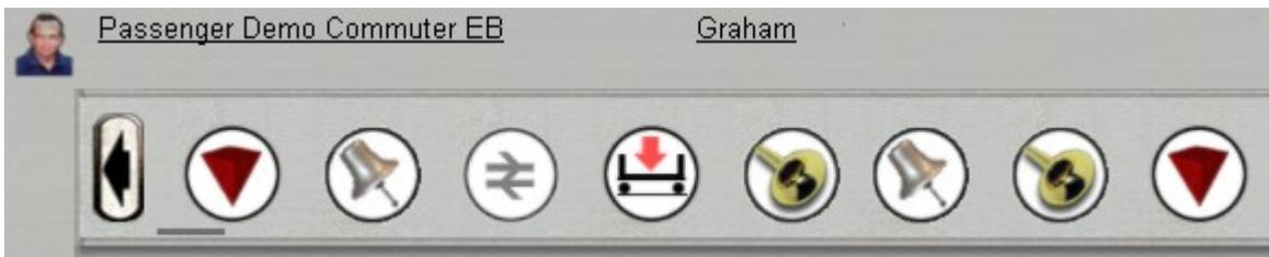
The first red trackmark tells the train to “Drive via Trackmark Pocono Bell EB”. As soon as the train hits the trackmark, it sees the Bellz command and the bell begins to ring. At same instant, the train sees the command to drive to the station and begins to slow down.
