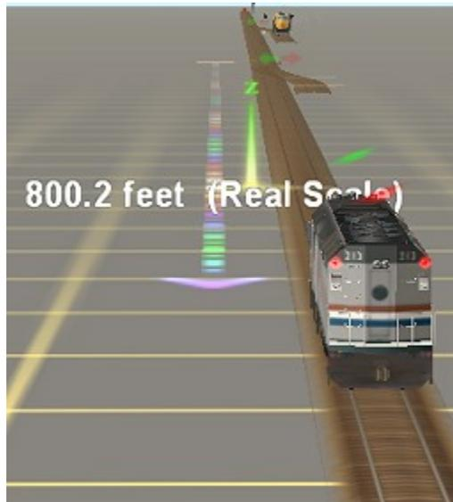
After experimenting a bit it seems that if the F40 is more than 800 feet/246m from the dummy switch when the GP38 starts, the GP38 can still leave the sidetrack. If the F40 is closer than that, the F40 will lock the turnout in front of the GP38 as well, forcing it to wait until the F40 has passed. Actually that seems pretty prototypical, for the sidetrack train to wait if the oncoming mainline train is reasonably close.
