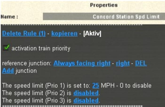
Now I've filled in the rest of dialog box, telling the control to watch junction "Always facing right" and whenever it's facing in the right hand direction—which it is always is—to set the speed limit for priority 1 trains to 25. What this does is set a continuous speed limit of 25 for all trains with a priority of 1.
