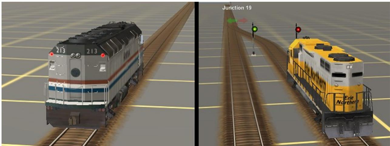
In the right-hand picture above we have a GP38 waiting to leave a sidetrack. The left picture is our oncoming mainline train, an Amtrak F40PH. Notice the turnout is aligned toward the mainline train and the F40 has a green signal. The GP38 has a stop signal.
